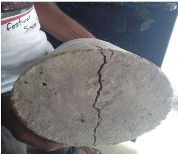
Fig.1 Split tensile crack
